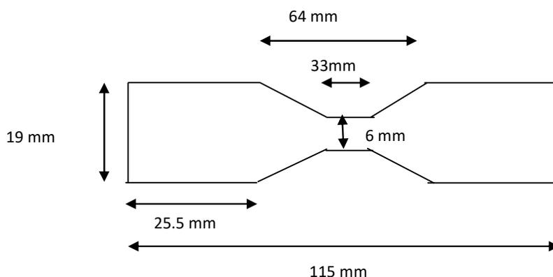
Figure 1. Specimen Tensile Strength Testing Based on ASTM D-638-72-Type IV
