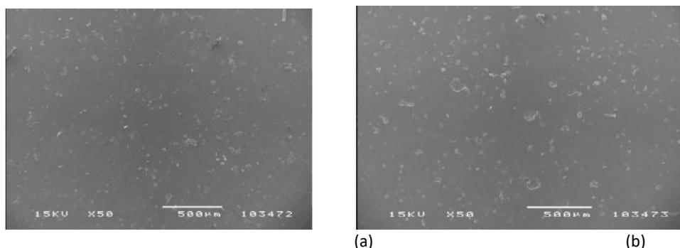
**Figure 3 Morphology of PU membrane from free fatty acid (a) before and (b) after reverse osmosis process**
