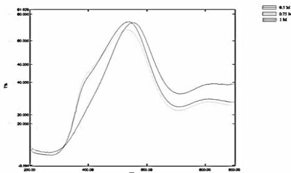
Figure 7. UV-Vis transmittance spectra of Cu<sub>2</sub>O nanoparticles.
