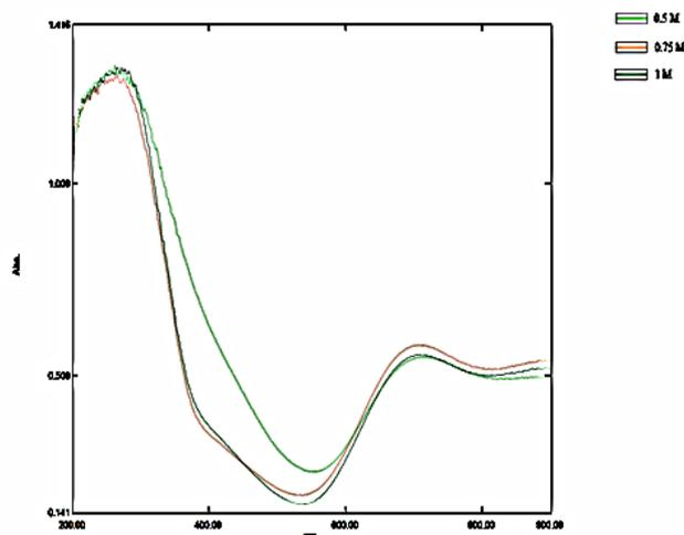
**Figure 5.** UV-Vis absorption spectra of  $\text{Cu}_2\text{O}$  nanoparticles.
