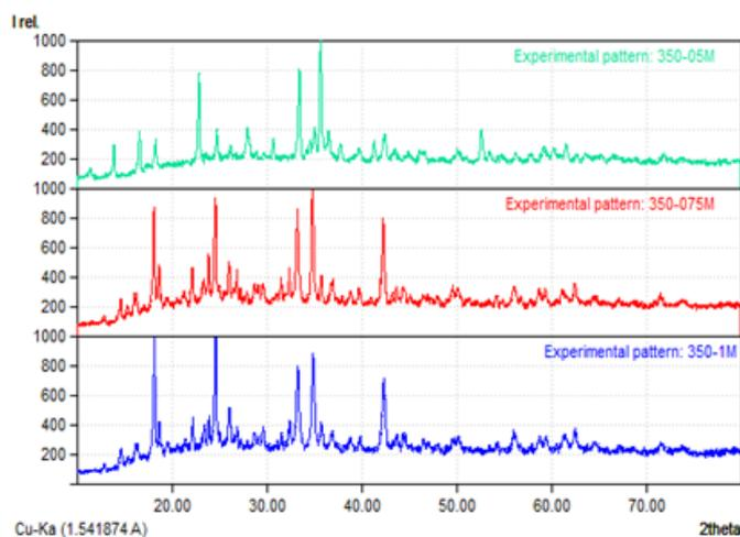
**Figure 2.** Powder XRD patterns of Cu<sub>2</sub>O nanoparticles by various concentration precipitator.
