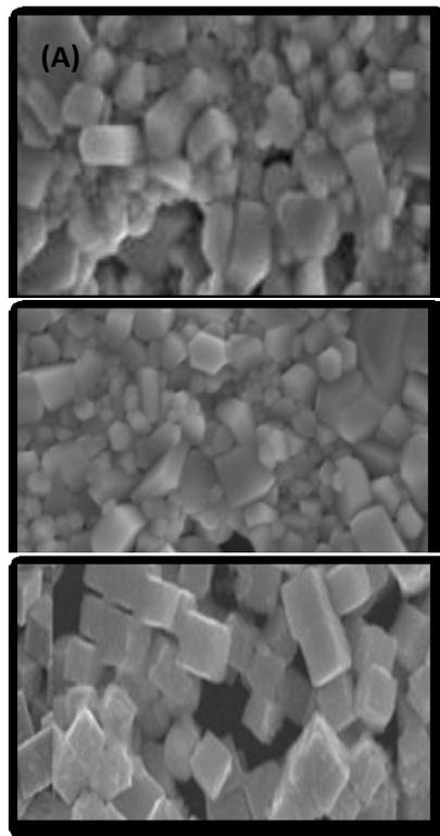
**Figure 4.** Typical SEM image of the  $\text{Cu}_2\text{O}$  nanoparticle by various concentration precipitator (a) 0.5 M, (b) 0.75 M, (c) 1 M
