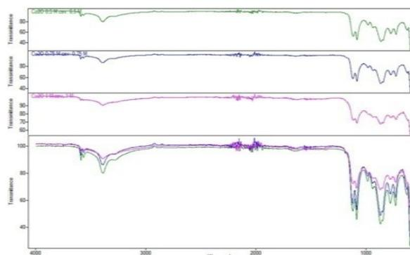
**Figure 1.** FTIR spectrum of Cu<sub>2</sub>O nanoparticles by various concentration precipitator.
