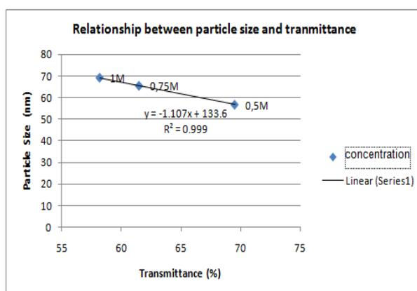
Figure 8. Relationship between particle size and transmittance
