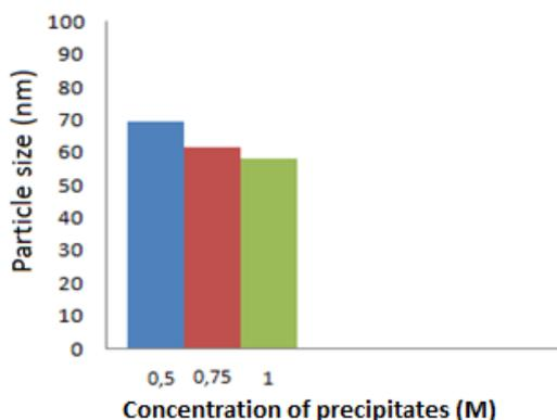
**Figure 3.** Relationship between pre cipitant concentration and particle size (based on Scherrer equation) of the  $\text{Cu}_2\text{O}$  nanocrystal.
