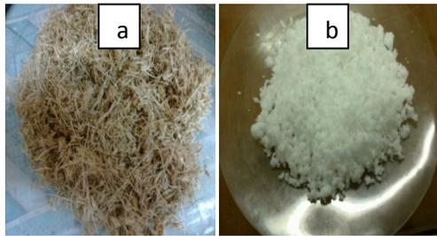
**Figure 1.** (a) The original of EFB fiber and (b) after bleaching
