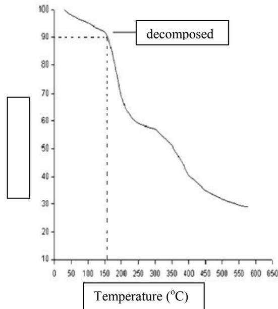
**Figure4.** TGA nanocrystalline cellulose from EFB
