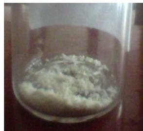
**Figure 2.** Nanocrystalline cellulose of palm empty fruit bunches
