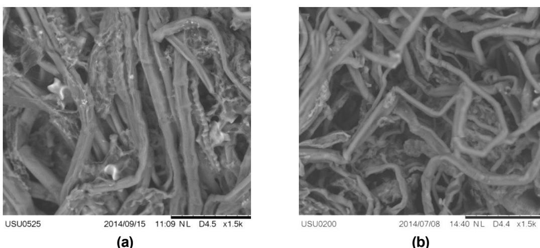
**Fig. 2.** SEM image of fiber before 17.5% NaOH treatment (a) dan  $\alpha$ -cellulose of rice leaves magnification 1500X)
