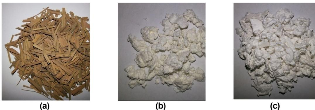
**Fig. 1** Dried rice leaves (a), fibers before 17.5% NaOH treatment (b),  $\alpha$ -cellulose rice leaves(c)
