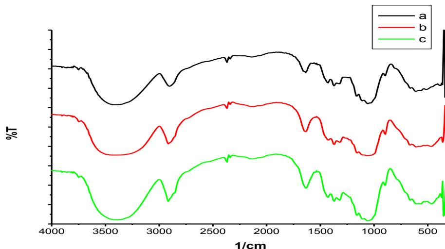
**Fig. 3.** FT-IR spectra of standard  $\alpha$ -cellulose d (a),  $\alpha$ -cellulose of rice leave (b), and fiber before 17.5% NaOH treatment (c)
